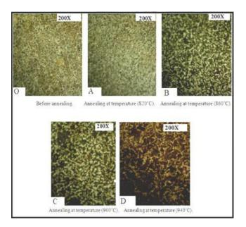
micro structure of carbon steel C45 before and after annealing at 200x.
