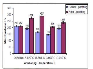
Micro hardness Hv Before Upsetting After Upsetting. Effect of upsetting process on the micro-hardness of low carbon steel C45 and its regimes.
